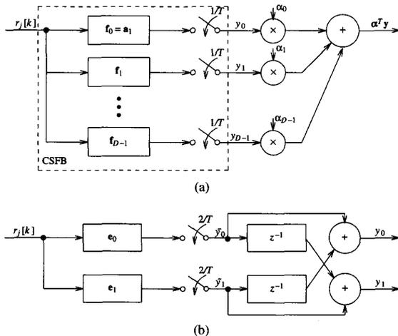
Fig. 2. (a) Detector with cyclically shifted filter bank.  $f_0, \dots, f_{D-1}$  are cyclic shifts of the matched filter  $a_1$ . (b) Reduced complexity CSFB for  $D = 2$ .
