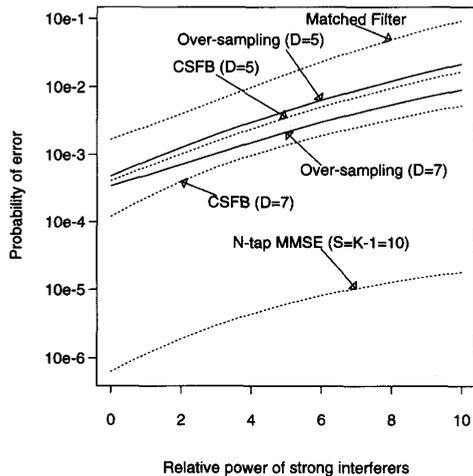
Fig. 6. Average error probability versus relative power of strong interferers. The parameters are the same as in Fig. 5.
