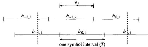
Fig. 3. Illustration of channel output samples  $r[k]$ , which are used to compute the estimated symbol  $b_{0,1}$ . The contribution to the channel output from the desired user and the  $j$ th interferer are shown. For the delay  $\tau_j$  shown in the figure, the estimate  $\hat{b}_{0,1}$  depends on the interference symbols  $b_{-1,j}$ ,  $b_{0,j}$ ,  $b_{1,j}$ , and  $b_{-1,1}$ .
