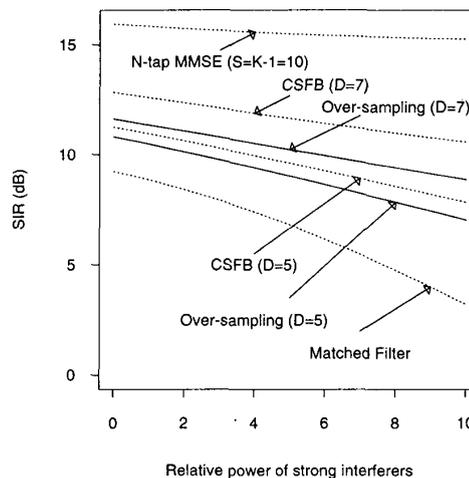
Fig. 5. SIR versus the relative power of strong interferers. For the  $N$ -tap MMSE detector ( $N = 31$ ),  $K = 11$  with 10 strong interferers, and for the simpler schemes,  $K = 5$  with two strong interferers.
