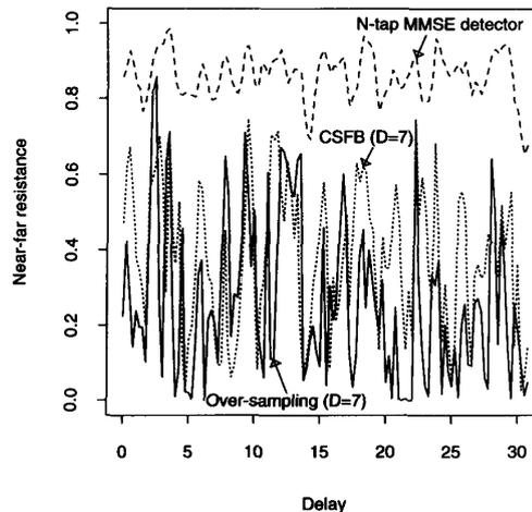
Fig. 4. Near-far resistance of MMSE detectors versus delay  $\nu_2$  ( $N = 31$ ,  $K = 3$ ).
