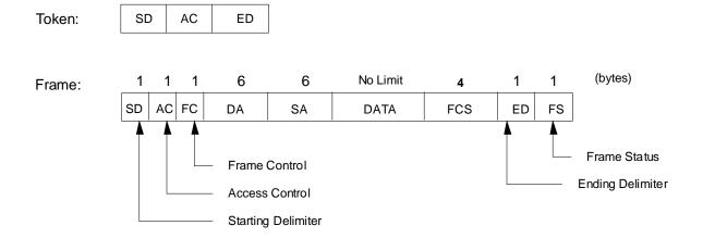
Note: while there is no explicit limit on the data field size, there is a maximum token holding time for any node, which implicitly limits the data field size.
