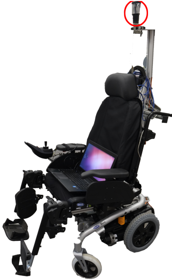
Fig. 3. The omnidirectional camera (circled in red) embedded on the wheelchair
